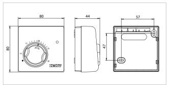
Electrical contact capacity = 16(2,5) A / 250 Vac Regulation range =  $5^{\circ} \div 30^{\circ}C$ Differential = 1K Insulation class = II Protection rating = IP20 Max. tolerance temperature = 50°C Connection = 2 wires Output = changeover switches Operating mode: On/Off or Summer/Winter System: heating/air conditioning Certifications: CE, ENEC03, EAC
